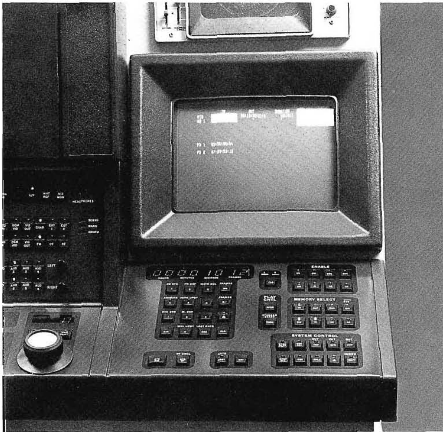
Local Control Panel for AE-800 Time Code Editing System
