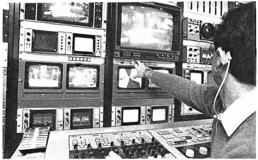
Set-up and remote controls for TK-47 cameras are located in Master Control.
