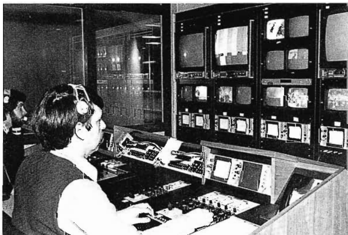
Video control for the two main studios are also identical. Camera controls for eight TK-47 cameras and two TK-760's are mounted in each of these video control consoles.
