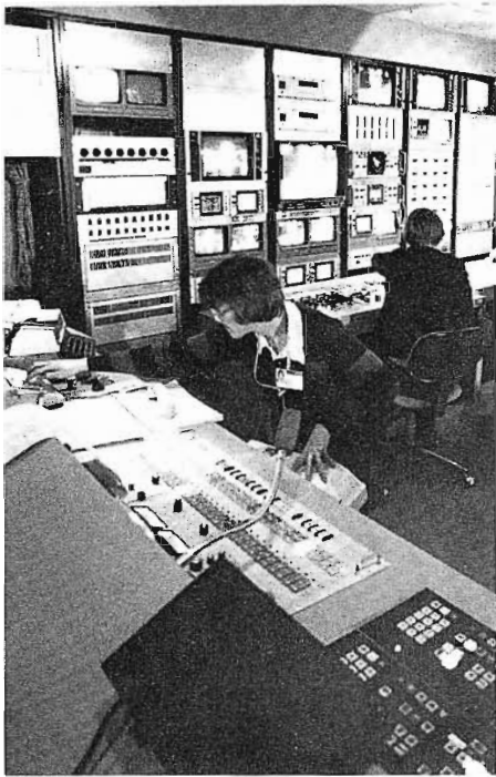
Master Control includes graphics, switching, camera control, satellite receiver controls and extensive monitoring facilities.
