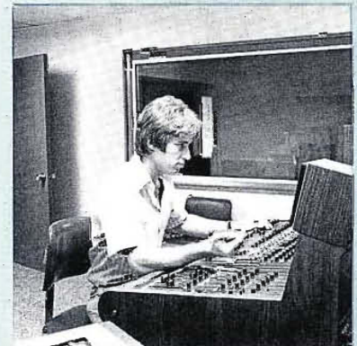
Audio quality and control is extremely important at Video Base. Complex mixes for video are handled through a time code interlock of audio and video tape recorders.
