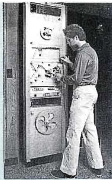
Threading an RCA PM-86SL, Tom Gasek prepares for a sound transfer session.
